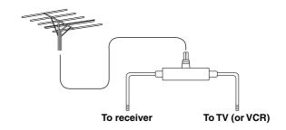
Connecting the antenna cable to the 75/300  $\Omega$  antenna adapter (For all models other than USA & Canadian models and European models)
